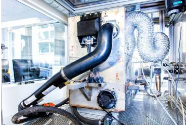
Figure 5:9 The test bench for Nissan's solid oxide fuel cell that runs on bio-ethanol electric power (Automotive News, 2016; photo by Nissan).
