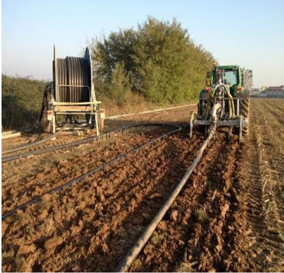
Figure 10 - Digestate is injected into the soil using an 'umbilical cord' to avoid soil compaction
