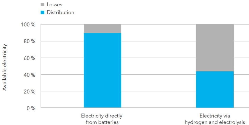
Figure 8. Comparison of energy losses when charging a battery compared with using electricity to produce hydrogen and run a fuel cell (DNV GL, 2015)
