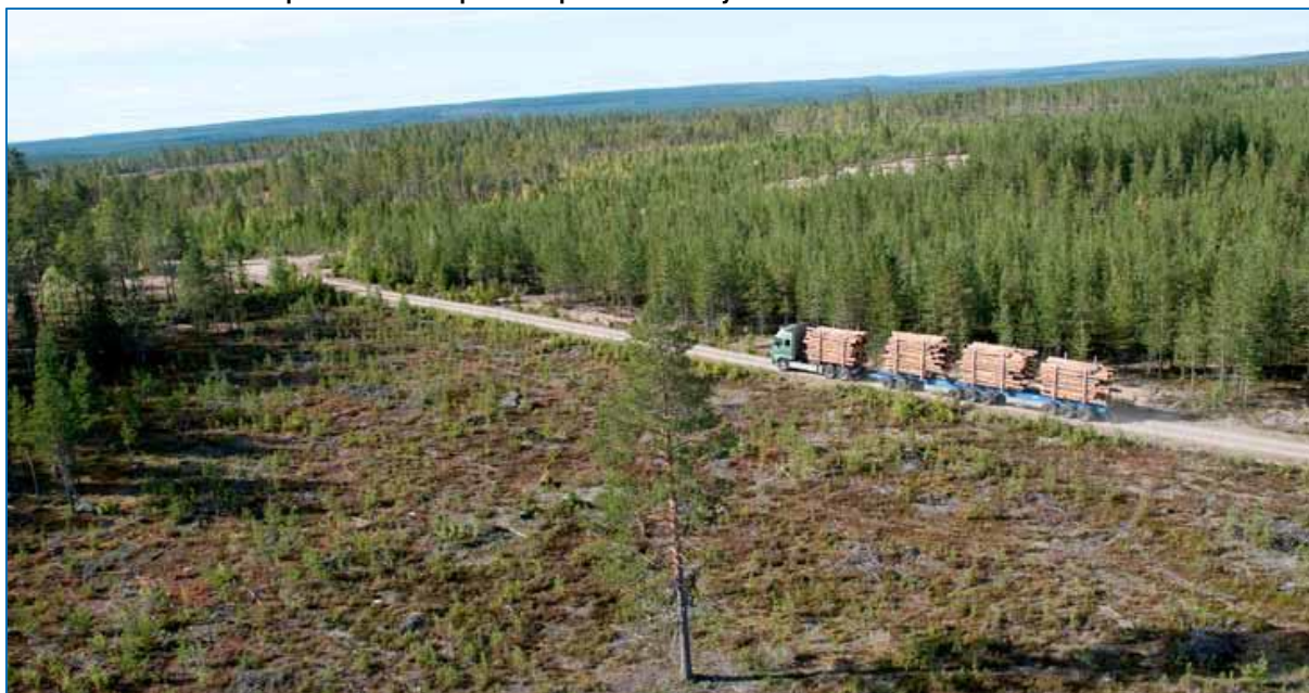
Figure 4.4 High Capacity Transport Trucks with a length of 25 to 30 m could reduce fuel consumption, GHG emissions and transportation costs per transported tonne by 10-20%
