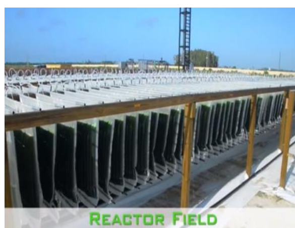
closed PBRs using patented VIPER technology, USA 19
