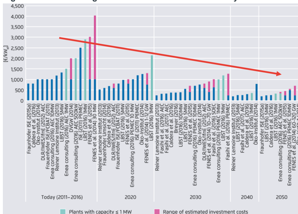
Figure 28 Decreasing investment cost for water electrolysis until 2050
