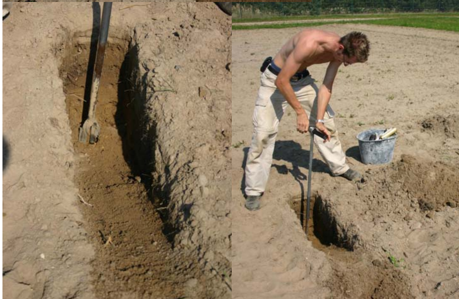
Fig 3.1.-4: From the bottom of the soilpit a hole will be bored to detect soil layering and a shallow watertable.
